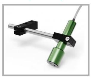
Type of projection: Cross Supply voltage: 9-36 Vdc 10-30 Vac Connection: Cable 2x0,25 cm 200 Light source: Laser diode Casing: Green anod.alum. Dimension: 20/30x110 mm Protection class: IP64 Storage temperature °C/°F: -40 +85 °C / -40 +185 °F Operating temperature °C/°F: -10 +50 °C / 14 +122 °F
