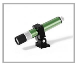
Type of projection: Cross Supply voltage: 9-36 Vdc 10-30 Vac Connection: M12 connector + cm 500 cable Light source: Laser diode Casing: Green anod.alum. Dimension: 20x135 mm Protection class: IP67 Storage temperature °C/°F: -40 +85 °C / -40 +185 °F Operating temperature °C/°F: -20 +60 °C / -4 +140 °F
