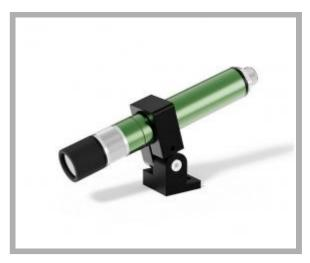
Type of projection: Circle Supply voltage: 9-36 Vdc 10-30 Vac Trigger 5-30Vdc Connection: M12 connector + cm 500 cable Light source: Laser diode Casing: Green anod.alum. Dimension: 20x135 mm Protection class: IP67 Storage temperature °C/°F: -40 +85 °C / -40 +185 °F Operating temperature °C/°F: -20 +60 °C / -4 +140 °F
