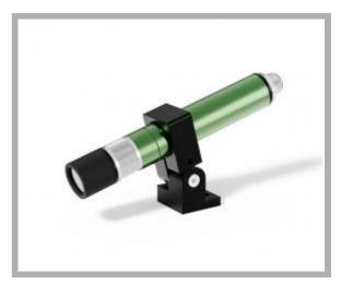
Type of projection: Line Supply voltage: 9-36 Vdc 10-30 Vac Connection: M12 connector + cm 500 cable Light source: Laser diode Casing: Green anod.alum. Dimension: 20x135 mm Protection class: IP67 Storage temperature °C/°F: -40 +85 °C / -40 +185 °F Operating temperature °C/°F: -20 +60 °C / -4 +140 °F
