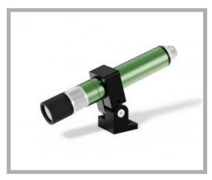
Type of projection: Circle Supply voltage: 9-36 Vdc 10-30 Vac Connection: M12 connector + cm 500 cable Light source: Laser diode Casing: Green anod.alum. Dimension: 20x135 mm Protection class: IP67 Storage temperature °C/°F: -40 +85 °C / -40 +185 °F Operating temperature °C/°F: -20 +60 °C / -4 +140 °F
