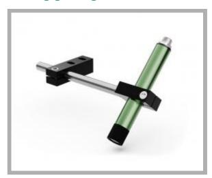
Type of projection: Line Supply voltage: 9-36 Vdc 10-30 Vac Trigger 5-30Vdc Connection: M12 connector + cm 500 cable Light source: Laser diode Casing: Green anod.alum. Dimension: 20x145 mm Protection class: IP67 Storage temperature °C/°F: -40 +85 °C / -40 +185 °F Operating temperature °C/°F: -20 +60 °C / -4 +140 °F
