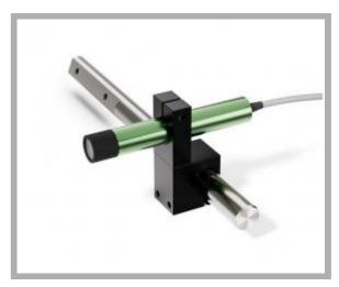
Type of projection: Circle Supply voltage: 9-36 Vdc 10-30 Vac Connection: Cable 2x0,25 cm 200 Light source: Laser diode Casing: Green anod.alum. Dimension: 20x130 mm Protection class: IP67 Storage temperature °C/°F: -40 +85 °C / -40 +185 °F Operating temperature °C/°F: -20 +60 °C / -4 +140 °F
