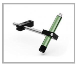
Type of projection: Cross Supply voltage: 9-36 Vdc 10-30 Vac Trigger 5-30Vdc Connection: M12 connector + cm 500 cable Light source: Laser diode Casing: Green anod.alum. Dimension: 20x145 mm Protection class: IP67 Storage temperature °C/°F: -40 +85 °C / -40 +185 °F Operating temperature °C/°F: -20 +60 °C / -4 +140 °F
