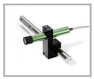
Type of projection: Dot Supply voltage: 9-36 Vdc 10-30 Vac Connection: Cable 2x0,25 cm 200 Light source: Laser diode Casing: Green anod.alum. Dimension: 20x130 mm Protection class: IP67 Storage temperature °C/°F: -40 +85 °C / -40 +185 °F Operating temperature °C/°F: -20 +60 °C / -4 +140 °F
