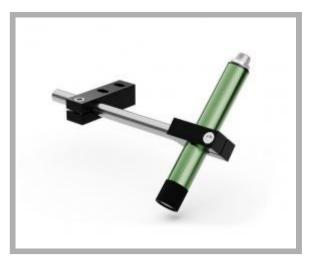
Type of projection: Dot Supply voltage: 9-36 Vdc 10-30 Vac Trigger 5-30Vdc Connection: M12 connector + cm 500 cable Light source: Laser diode Casing: Green anod.alum. Dimension: 20x145 mm Protection class: IP67 Storage temperature °C/°F: -40 +85 °C / -40 +185 °F Operating temperature °C/°F: -20 +60 °C / -4 +140 °F
