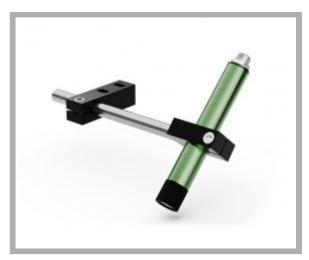
Type of projection: Dot Supply voltage: 9-36 Vdc 10-30 Vac Connection: M12 connector + cm 500 cable Light source: Laser diode Casing: Green anod.alum. Dimension: 20x145 mm Protection class: IP67 Storage temperature °C/°F: -40 +85 °C / -40 +185 °F Operating temperature °C/°F: -20 +60 °C / -4 +140 °F
