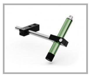
Type of projection: Circle Supply voltage: 9-36 Vdc 10-30 Vac Connection: M12 connector + cm 500 cable Light source: Laser diode Casing: Green anod.alum. Dimension: 20x145 mm Protection class: IP67 Storage temperature °C/°F: -40 +85 °C / -40 +185 °F Operating temperature °C/°F: -20 +60 °C / -4 +140 °F
