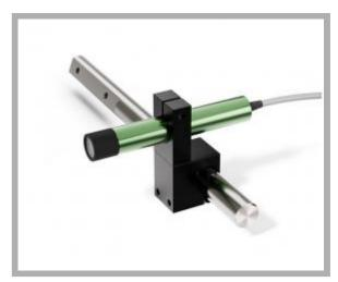
Type of projection: Line Supply voltage: 9-36 Vdc 10-30 Vac Connection: Cable 2x0,25 cm 200 Light source: Laser diode Casing: Green anod.alum. Dimension: 20x130 mm Protection class: IP67 Storage temperature °C/°F: -40 +85 °C / -40 +185 °F Operating temperature °C/°F: -20 +60 °C / -4 +140 °F
