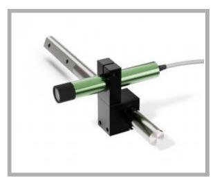
Type of projection: Cross Supply voltage: 9-36 Vdc 10-30 Vac Connection: Cable 2x0,25 cm 200 Light source: Laser diode Casing: Green anod.alum. Dimension: 20x130 mm Protection class: IP67 Storage temperature °C/°F: -40 +85 °C / -40 +185 °F Operating temperature °C/°F: -20 +60 °C / -4 +140 °F
