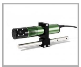
Type of projection: Perpendicular line exit Supply voltage: 80-265 Vac Connection: Cable 3x0,75 cm 300 with schuco plug Light source: Laser diode Casing: Green anod.alum. Dimension: 50X250 mm Protection class: IP64 Storage temperature °C/°F: -40 +85 °C / -40 +185 °F Operating temperature °C/°F: -20 +60 °C / -4 +140 °F
