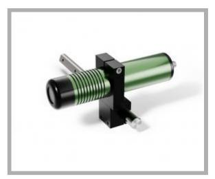
Type of projection: Line Supply voltage: 9-36 Vdc 10-30 Vac Trigger 5-30Vdc Connection: M12 connector + cm 500 cable Light source: Laser diode Casing: Green anod.alum. Dimension: 50X230 mm Protection class: IP67 Storage temperature °C/°F: -40 +85 °C / -40 +185 °F Operating temperature °C/°F: -20 +60 °C / -4 +140 °F
