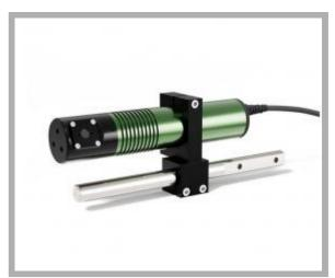
Type of projection: Perpendicular line exit Supply voltage: 80-265 Vac Connection: Cable 3x0,75 cm 300 without plug Light source: Laser diode Casing: Green anod.alum. Dimension: 50X250 mm Protection class: IP64 Storage temperature °C/°F: -40 +85 °C / -40 +185 °F
