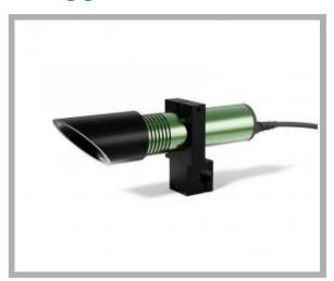
Type of projection: Line Supply voltage: 80-265 Vac Connection: Cable 3x0,75 cm 300 without plug Light source: Laser diode Casing: Green anod.alum. Dimension: 50X220 mm Protection class: IP67 Storage temperature °C/°F: -40 +85 °C / -40 +185 °F Operating temperature °C/°F: -10 +50 °C / 14 +122 °F
