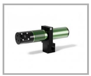
Type of projection: Perpendicular line exit Supply voltage: 9-36 Vdc 10-30 Vac Connection: M12 connector + cm 500 cable Light source: Laser diode Casing: Green anod.alum. Dimension: 50X255 mm Protection class: IP64 Storage temperature °C/°F: -40 +85 °C / -40 +185 °F Operating temperature °C/°F: -10 +50 °C / 14 +122 °F
