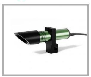
Type of projection: Line Supply voltage: 80-265 Vac Connection: Cable 3x0,75 cm 300 with schuco plug Light source: Laser diode Casing: Green anod.alum. Dimension: 50X220 mm Protection class: IP67 Storage temperature °C/°F: -40 +85 °C / -40 +185 °F Operating temperature °C/°F: -10 +50 °C / 14 +122 °F
