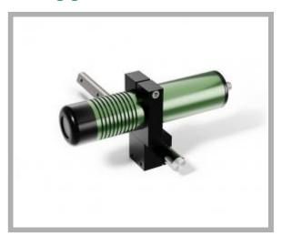
Type of projection: Line Supply voltage: 9-36 Vdc 10-30 Vac Trigger 5-30Vdc Connection: M12 connector + cm 500 cable Light source: Laser diode Casing: Green anod.alum. Dimension: 50X230 mm Protection class: IP67 Storage temperature °C/°F: -40 +85 °C / -40 +185 °F Operating temperature °C/°F: -10 +50 °C / 14 +122 °F
